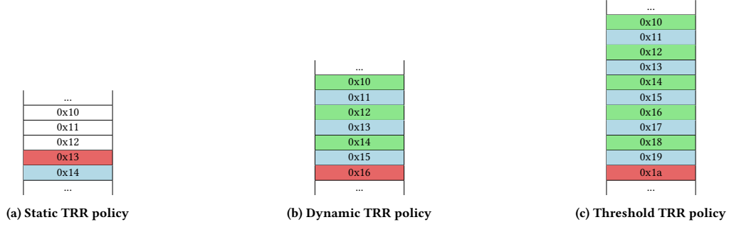
Figure 3: Example TRR policies. Grey rows are potential aggressor rows, green ones are potential victims that are refreshed by TRR, and red ones are victim rows.
